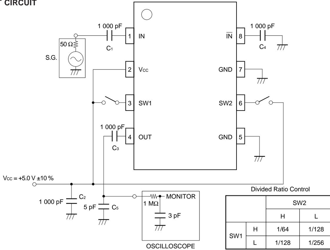
ILLUSTRATION OF TEST CIRCUIT ASSEMBLED ON EVALUATION BOARD
