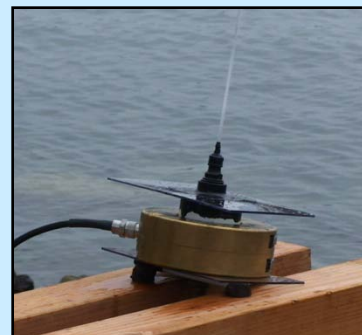
A stream of salt water can be used to transmit and receive signals over various frequencies and bandwidths.
