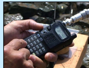
The patented antenna has been tested at a distance of over 30 miles at frequencies ranging from 2 to 400 MHz.
